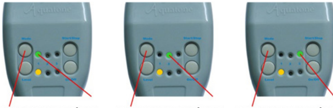
Install the modulation mode by cyclic touch of Mode button Mode 1 Mode 2 Mode 3
