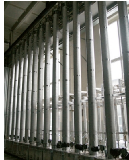
Current Manufacturing process of Lightwater (Vacuum Fractional distillation–rectification)
